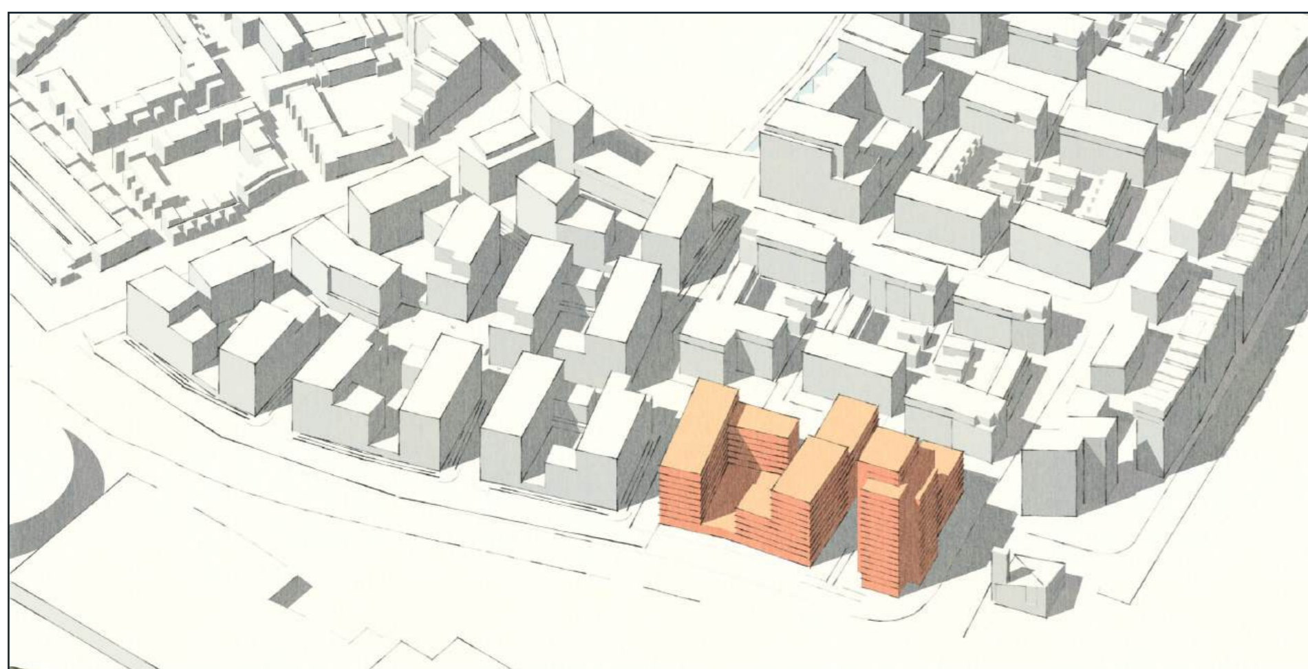
TWO BLOCKS APPROACH WITH A LINEAR BLOCK TO THE EASTERN END TO PROVIDE ACOUSTIC BUFFER FROM THE WHARF OPERATIONS
